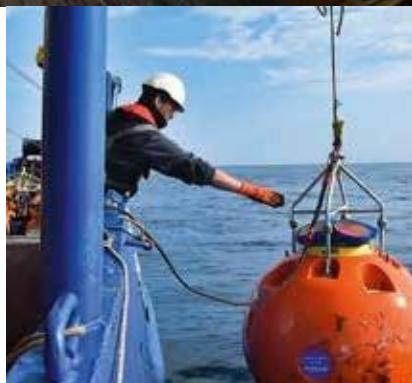
Lifting of a buoy station which measures the hydrological parameters of water for an upload of measurement data and battery replacement
