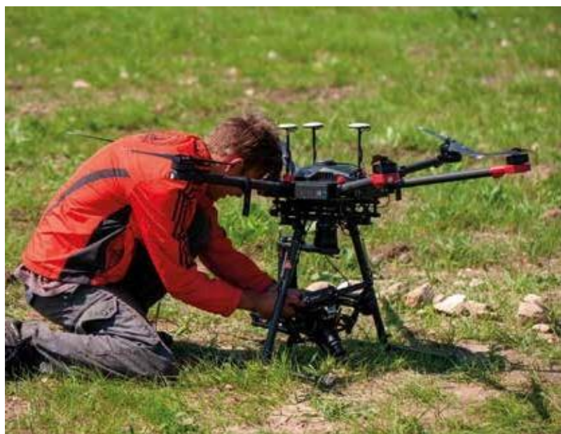
Preparing a UAV for shooting with a hyperspectral camera
